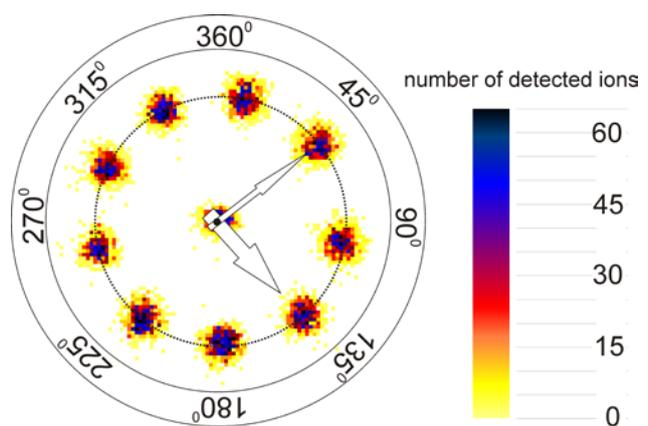
Fig. 2. Radial movement of the ion on the detector (“Phase watch”) for different stopping times. The figure is composed of a great number of single measurements which could be taken within some minutes. The rotating moment of the ion is approximately 1 microsecond.
