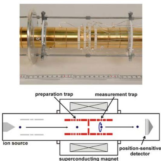
Fig. 1. Schematic of the setup of the SHIPTRAP trap with a space resolving detector for imaging the radial motion of the ion.
